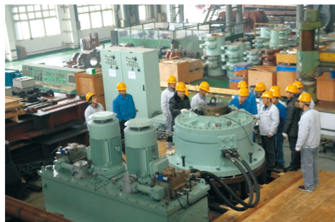
舵机负载试验 Load Test of Rotary Vane Steering Gear
