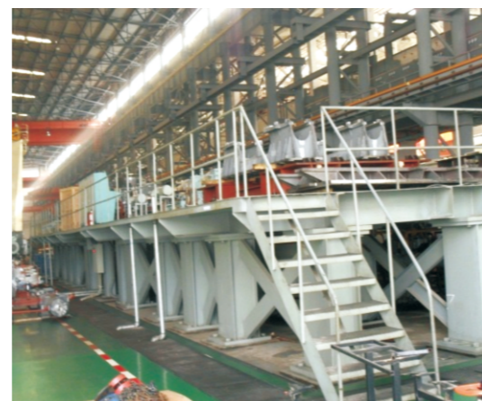
2x3000kNm大型舵机综合试验台 Complex Test Bed for large Steering Gear
